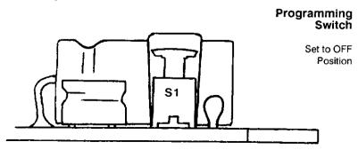
The programming switch is activated (turned ON), by pushing the switch actuator downwards. To turn the switch OFF, lift the actuator upwards with a fingernail. The direction of movement to turn the switch ON is marked on one side of the switch body.
