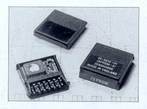
An Erasable Programmable Read Only Memory Module for the HP-41 Handheld Computer
