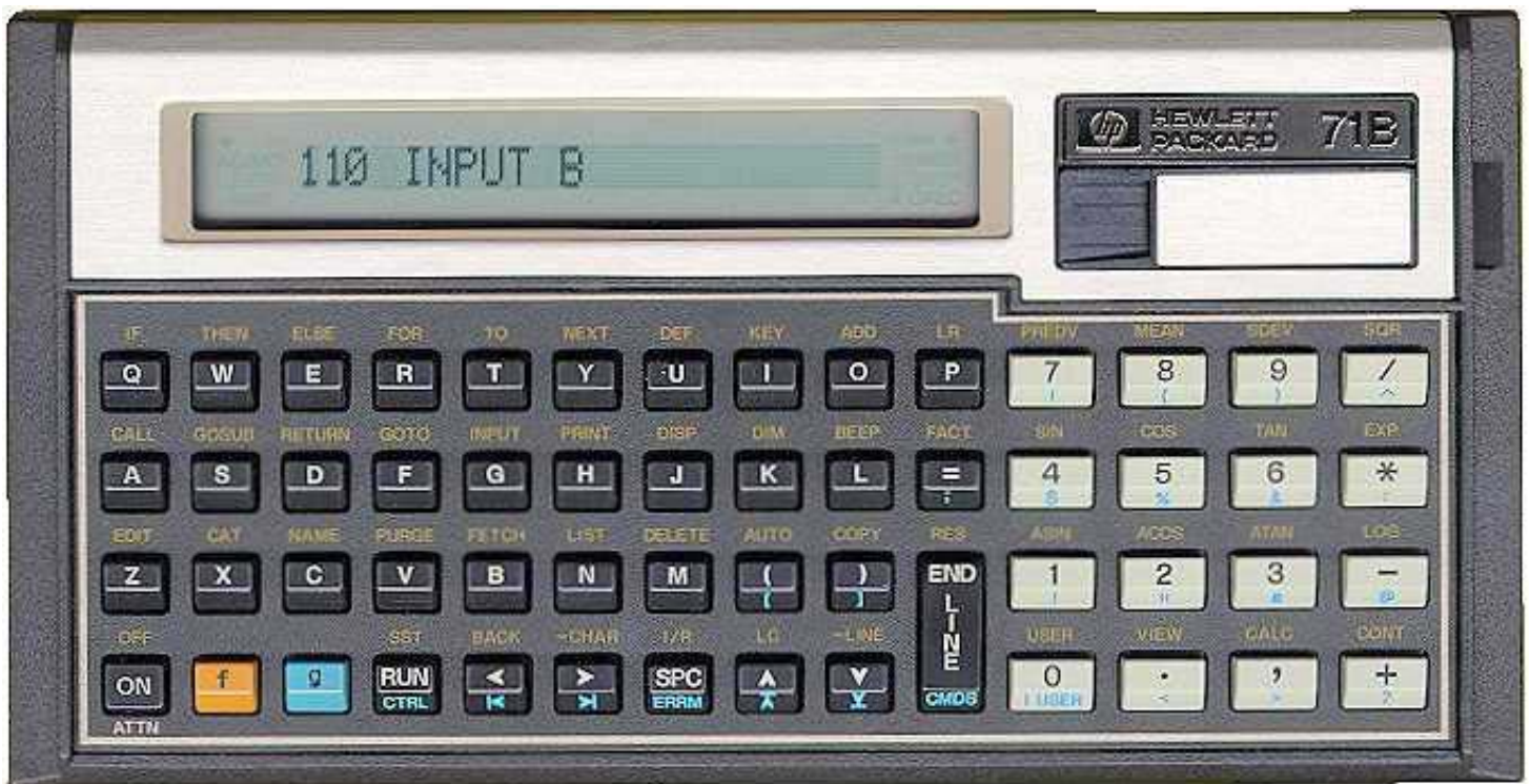
The HP-71B, shown full size with hand pulled card reader module, was introduced February 1, 1984.
