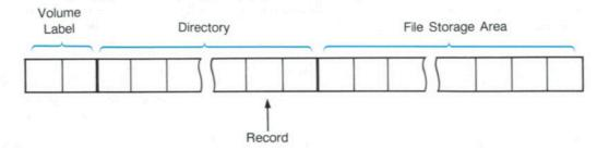
Each record (or "sector") on the medium consists of 256 eight-bit bytes, numbered 0 through 255.
