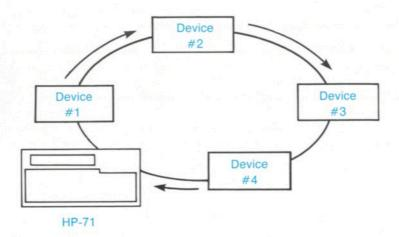
If any device isn't turned on, it will probably disrupt the operation of the HP-IL system because it can't pass messages around the loop.
