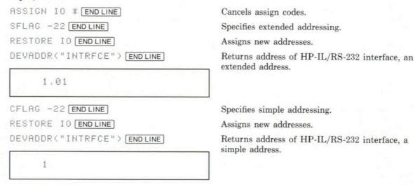
Three statements always cause the HP-71 to assign new addresses to HP-IL devices: ASSIGN IO, RESTORE IO, and CONTROL ON. The HP-71 uses flag -24 to control whether the HP-71 assigns new addresses at other times:
