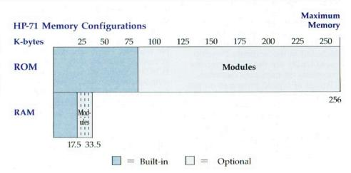
Any combination of up to four ROM and/or RAM modules may be inserted, to a maximum of 256K bytes of memory.
