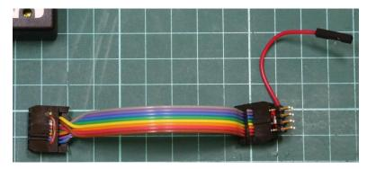
On the CN5-side of the cable, a 4 x 2 pin long male header is inserted into the cable's socket. A red wire with a single pole connector is connected to pins 3 and 5.
