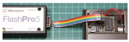
In order to conserve the HP-71B's batteries, FRAM71 doesn't supply VJTAG and VPUMP to the JTAG interface. Thus, when using FLashPro programmers, VJTAG
